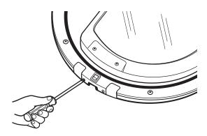
Remove the window retainer and set it aside. The window retainer is located on the side opposite the hinge assembly and underneath the plastic cover.
